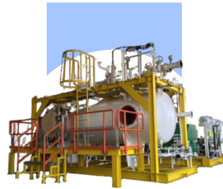
Flare Gas Liquid Compressor System
